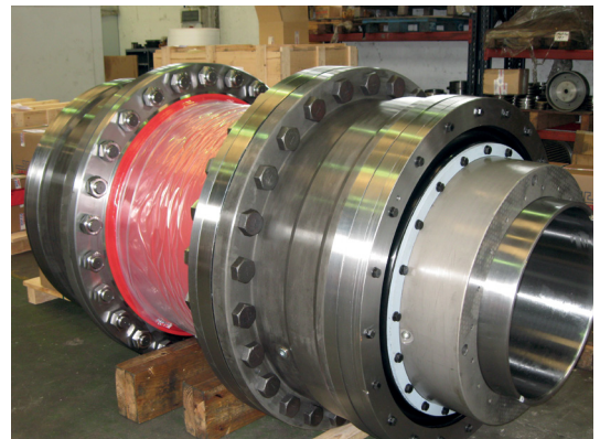
Dredger gear coupling
