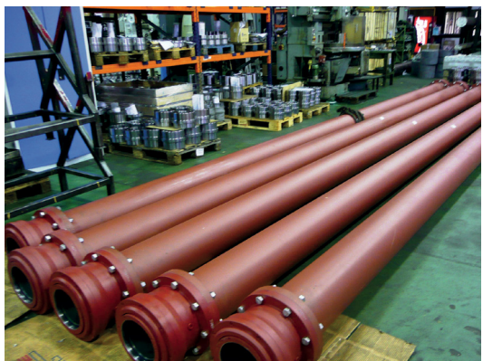
Jaure gear coupling for underwater operation
