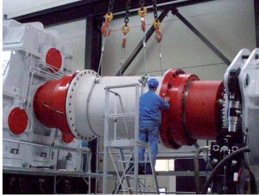
Jaure™ MTGX-HD-TI-1000/JHC-700 on wind test bench
