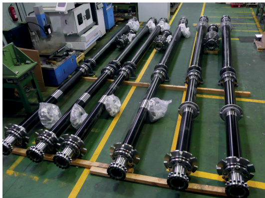
LAMIDISC coupling 380-8 JHSS with hollow steel spacer and bearings
