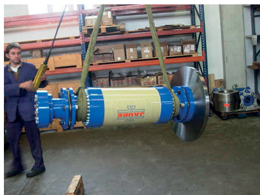
LAMIDISC coupling with JGFS glass fiber shaft for wind industry
