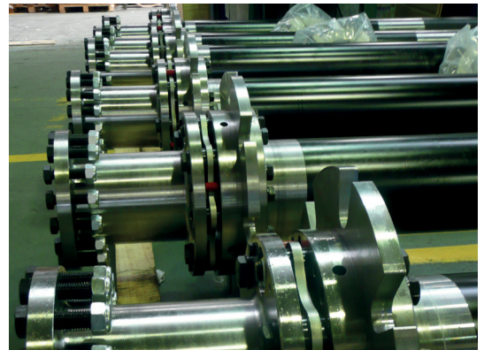
LAMIDISC coupling 410-8 with locking device
