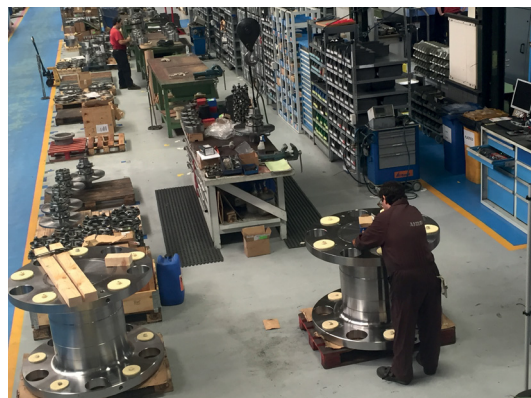
LAMIDISC coupling 1150-10 for marine propulsion
