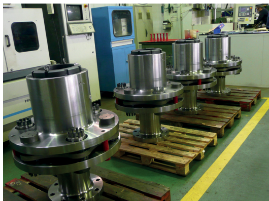
LAMIDISC coupling SU-JS-730-6-JHC-230 with hydraulic coupling
