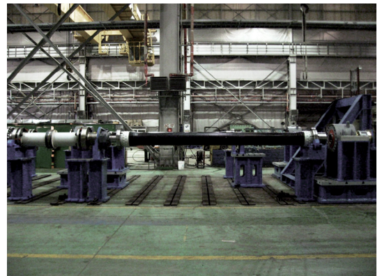
LAMIDISC coupling 605-8 with JCFS composite shafts
