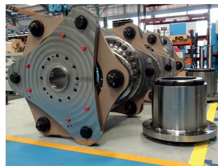
LAMIDISC coupling 1300-6 in combination with JHC-HF-320
