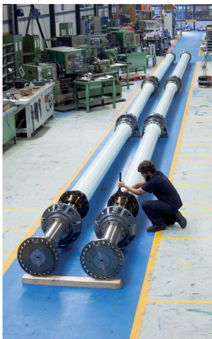
LAMIDISC™ coupling 505-8 with JCFS-FP Composite Shafts
