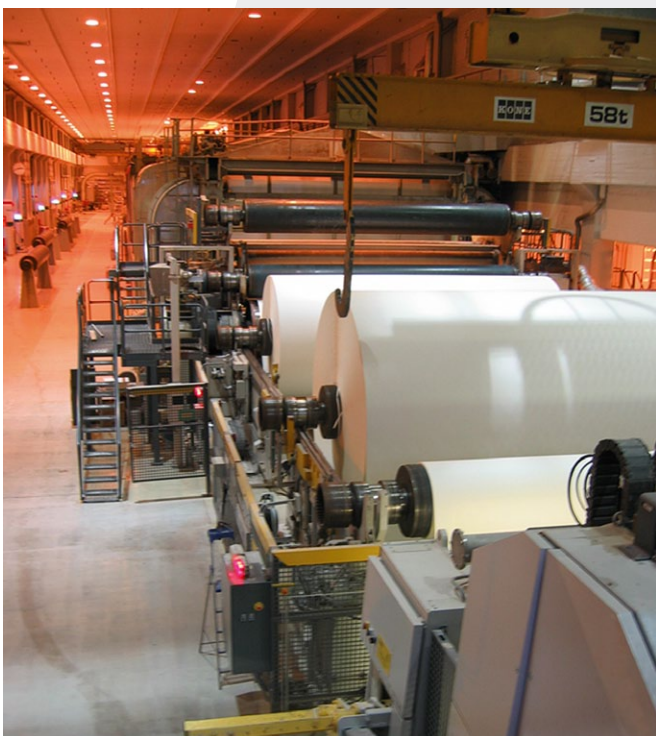
New Generation Yankee cylinder drive
