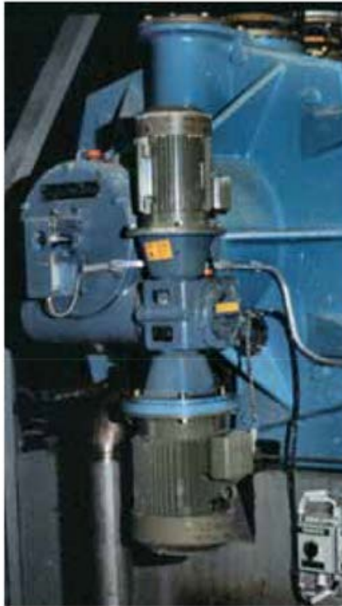
Covera loading device for low consistency refiner. Covera Schneckengetriebe in der Refiner-Spaltregelung.
